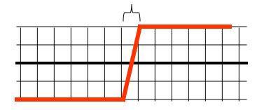
Output signal has a ramping factor.
