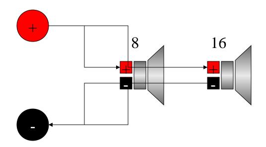
$$R_{t} = \frac{R_{1} \cdot R_{2}}{R_{1} + R_{2}}$$
