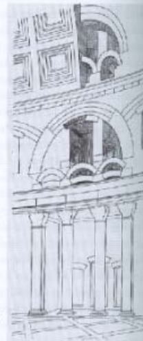
180 Pantheon. (Analytical drawing of structure after L. Beltrami)
