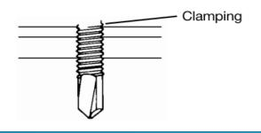
Thinner base material requires a coarser thread pitch to assure proper clamping. The thicker the material, the finer the threads must be. In very thick metal (3/8" to 1/2" thick), a fine thread is advisable. This will allow the thread to tap into the base material with less installation torque than a coarse thread.
