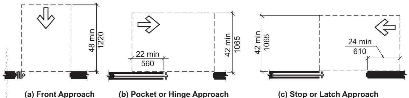
**FIG. 404.2.3.3 MANEUVERING CLEARANCE AT SLIDING AND FOLDING DOORS**
