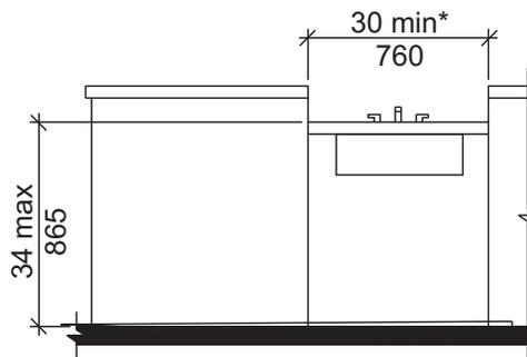
\* 36 min. (915) if part of T-shaped turning space per Sections 304.3.2 and 1003.3.2
