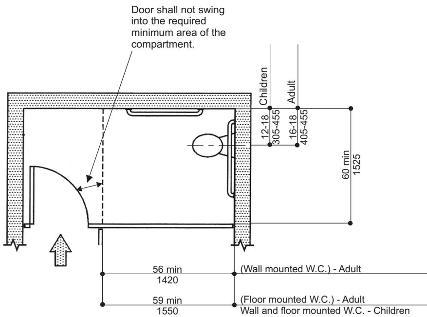
**FIG. 604.9.3.1 (C) WHEELCHAIR ACCESSIBLE COMPARTMENT DOOR OPENINGS—ALTERNATE**
