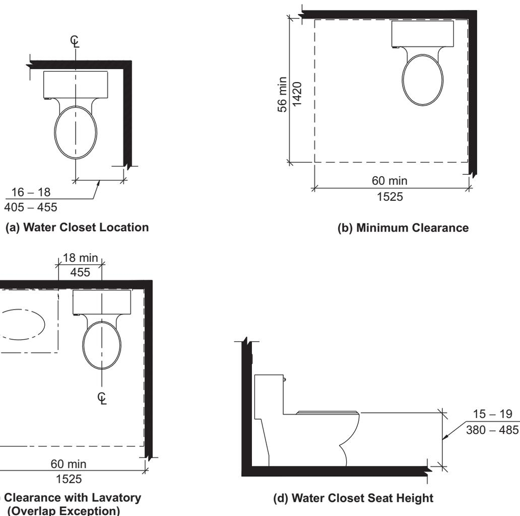
**FIG. 1003.11.2.4 WATER CLOSETS IN TYPE A UNITS**
