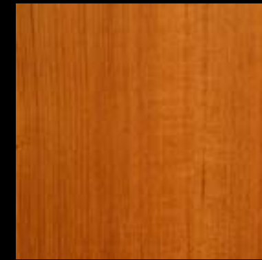
CABINETS (WDP02) Wood Veneer, Quarter Cut Afromosia, Clear Conversion Varnish
