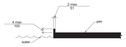
FIGURE 1103.3.1(C) (EXCEPTION 2) EDGE PROTECTION AT BOAT SLIPS
