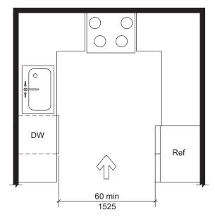
FIG. 1003.12.1.2 U-SHAPED KITCHEN CLEARANCE IN TYPE A UNITS
