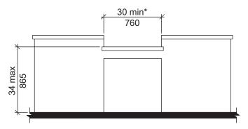
\* 36 min. (915) if part of T-shaped turning space per Sections 304.3.2 and 1003.3.2
