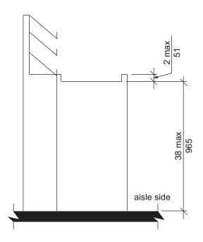
FIG. 904.4.2 HEIGHT OF CHECKOUT COUNTERS
