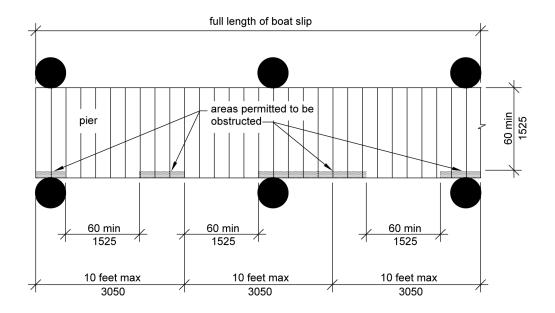
FIGURE 1103.3.1(A) BOAT SLIP CLEARANCE
