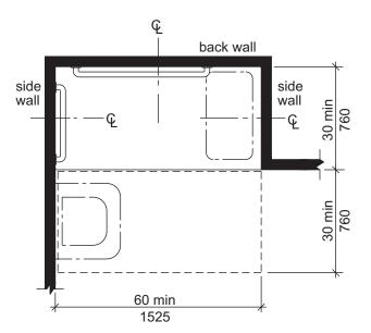
Note: inside finished dimensions measured at the center points of opposing sides
