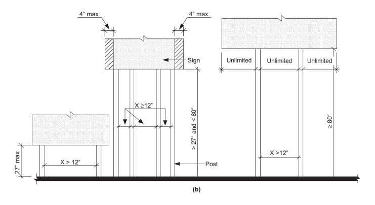
Fig. 307.3 Post-Mounted Protruding Objects
