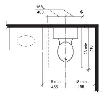
FIG. 1004.11.1.1 SWING-UP GRAB BAR FOR WATER CLOSET
