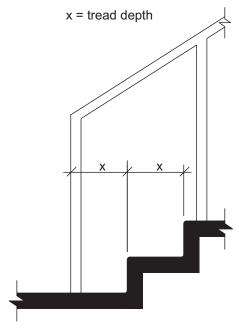
FIG. 505.10.3 BOTTOM HANDRAIL EXTENSIONS AT STAIRS
