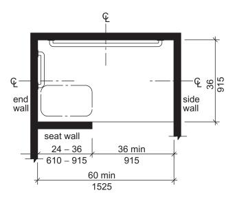
Note: inside finished dimensions measured at the center points of opposing sides
