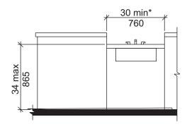
\* 36 min. (915) if part of T-shaped turning space per Sections 304.3.2 and 1003.3.2
