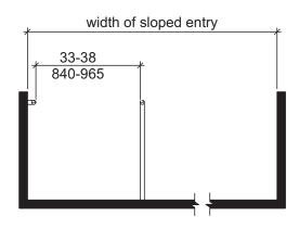
FIGURE 1109.3.3 HANDRAILS FOR SLOPED ENTRY
