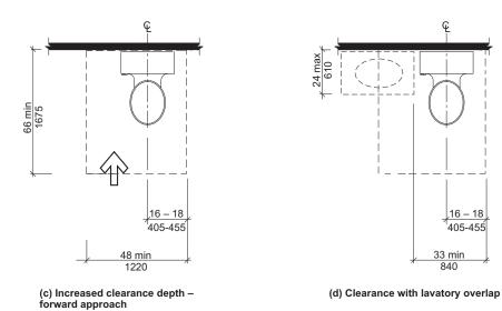
FIG. 1004.11.3.1.2 CLEARANCE AT WATER CLOSETS IN TYPE B UNITS
