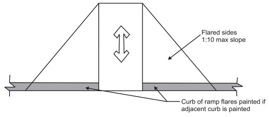
FIG. 406.3 SIDES OF CURB RAMPS
