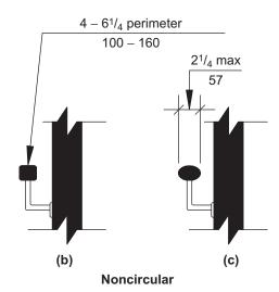
FIG. 505.7 HANDRAIL CROSS SECTION
