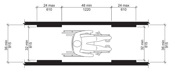
FIG. 403.5 CLEAR WIDTH OF AN ACCESSIBLE ROUTE
