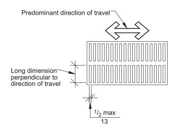
FIG. 302.3 OPENINGS IN FLOOR SURFACES
