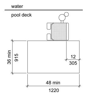
FIGURE 1109.2.3 CLEAR DECK SPACE AT POOL LIFTS
