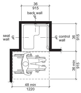
Note: inside finished dimensions measured at the center points of opposing sides
