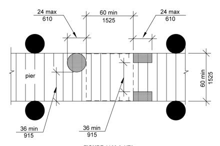
FIGURE 1103.3.1(B) (EXCEPTION 1) CLEAR PIER SPACE REDUCTION AT BOAT SLIPS
