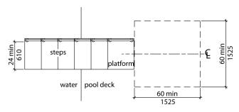
FIG. 1109.5.2 CLEAR DECK SPACE AT TRANSFER PLATFORM
