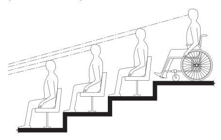
FIG. 802.9.1.1 LINES OF SIGHT OVER THE HEADS OF SEATED SPECTATORS
