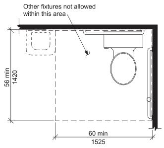
FIG. 604.3 SIZE OF CLEARANCE FOR WATER CLOSET
