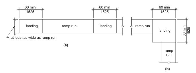
FIG. 405.7 RAMP LANDINGS **405.9 Edge Protection.** Edge protection complying with Section 405.9.1 or 405.9.2 shall be provided on each side of ramp runs and at each side of ramp landings.
