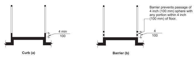
FIG. 405.9.2 RAMP EDGE PROTECTION
