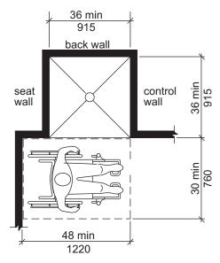
FIG. 1004.11.3.1.3.3 TRANSFER-TYPE SHOWER COMPARTMENT IN TYPE B UNITS
