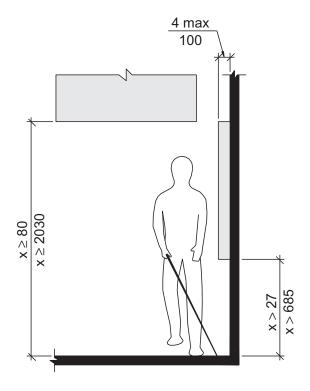
FIG. 307.2 LIMITS OF PROTRUDING OBJECTS
