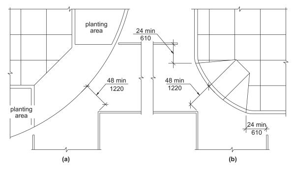
FIG. 406.10 DIAGONAL CURB RAMPS
