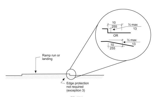
FIG. 405.9 EDGE PROTECTION—LIMITED DROP OFF
