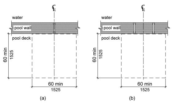
FIGURE 1109.4.1 CLEAR DECK SPACE AT TRANSFER WALLS
