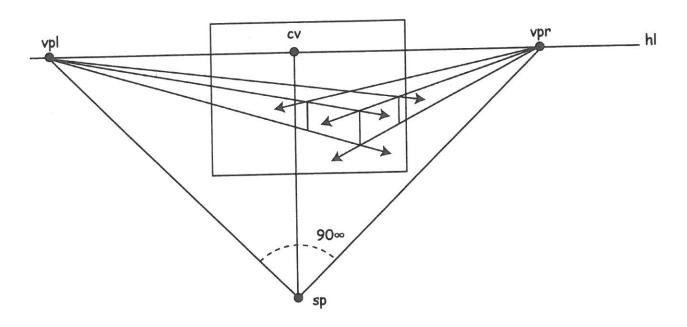
You can use the Center of Vision (cv) as 1pt perspective Vanishing Point (vp). You can make multiple 2pt perspectives by creating additional sets of vanishing points (vp1 & vp2) as long as they are  $90\infty$  from the Station Point (sp).
