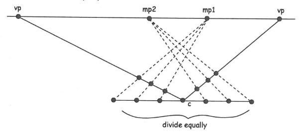
From these equal measurement points, connect lines to vanishing points.
