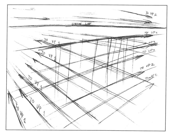
Two-Point Direct Drawing, Step 1- Perspective Grid
