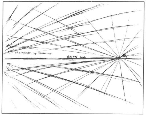
It is acceptable to put one of the vanishing points inside the composition, as long as it is not so much to the middle of the composition.
