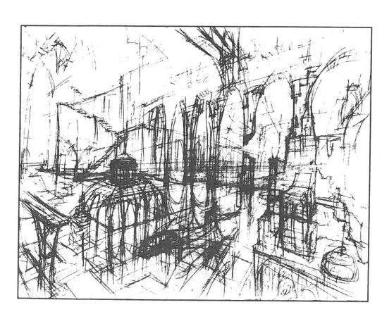
Notice that the right side area of the drawing, near the vanishing point is slightly distorted. This is acceptable because the distortion area does not cover a large space.
