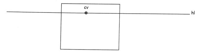
Draw a line straight down from your cv to some point below your drawing, where you end it is your Station Point (sp). Use the  $90\infty$  angle on your triangle from the Station Point, and draw lines out toward the Horizon Line, where they cross the Horizon Line determines your left and right Vanishing Points (vpl & vpr).
