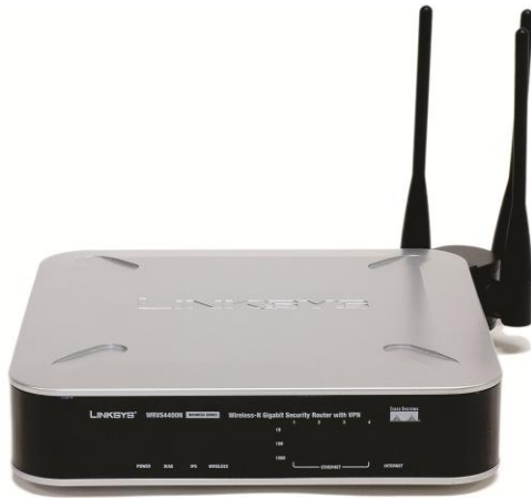
Figure 5: Linksys device that acts as wireless access point, switch, and router
