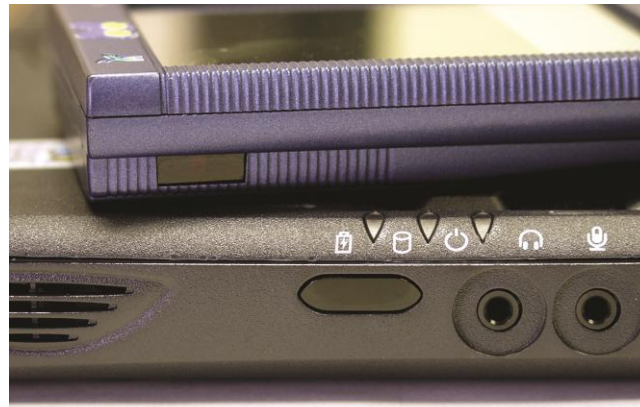
Figure 1: Infrared transceiver ports on a laptop and PDA
