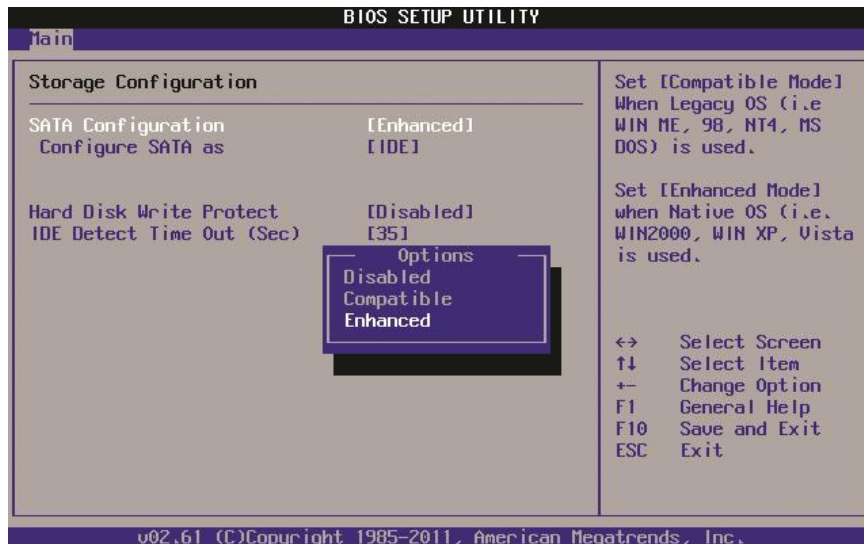
Figure 44: Typical controller settings in CMOS
