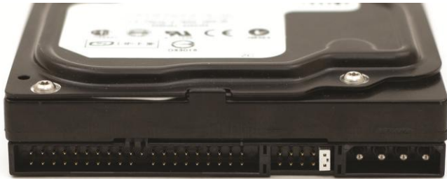
Figure 8: Back of IDE drive showing 40-pin connector (left), jumpers (center), and power connector (right)
