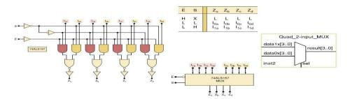
1. To ease the design process for commonly used system, such as adders, the Quartus II provide a build-in **Library of Parameterized Modules (LPM)**. For example, the *bdf* file can utilize four two-input multiplexer *lpm\_mux* module.
