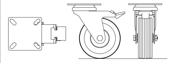
Notes: Swivel Casters should be 2-1/2" tall and compared to the dimension of and duty rating of the frame. For attaching the swivel casters on the projector, use Philips steel flat head screws 1",  $\frac{3}{16}$ "hexbolts,  $\frac{1}{2}$ " fasteners.
