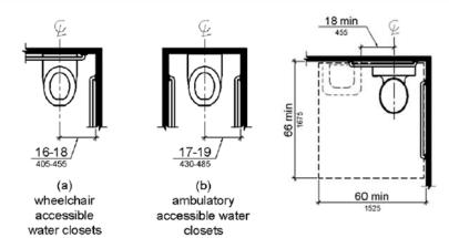
604.3.1 Size. Clearance around a water closet shall be 60 inches (1525 mm) minimum measured perpendicular from the side wall and 56 inches (1420 mm) minimum measured perpendicular from the rear wall.
