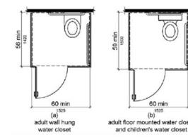
All Loading areas shall comply with a width of 36: in order for any person with a disability to rotate in a wheelchair 60" must be available in any landing due to ADA restrictions. For example elevators, ramps, doors, bathroom door swings, and entrances/exits.
