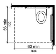
604.5.1 Side Wall. The side wall grab bar shall be 42 inches (1065 mm) long minimum, located 12 inches (305 mm) maximum from the rear wall and extending 54 inches (1370 mm) minimum from the rear wall.
