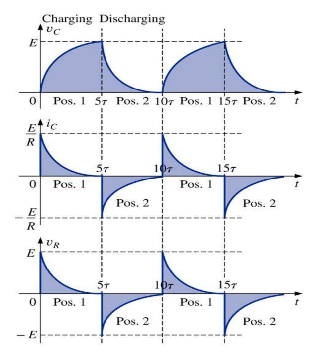
**Example9:** After  $v_C$  in Example 8 has reached its final value of 40 V, the switch is shown into position 2. Find the mathematical expressions for the transient behavior of  $v_C$ ,  $i_C$ , and  $v_R$  after the closing of the switch. Plot the curves for  $v_C$ ,  $i_C$ , and  $v_R$  using the defined directions and polarities in example 8. Assume that t = 0 when the switch is moved to position 2.
