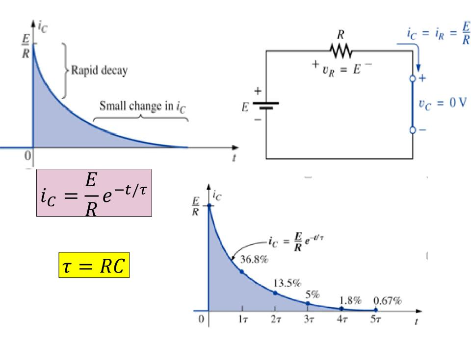
**Example8:** (a) Find the mathematical expressions for the transient behavior of  $v_C$ ,  $i_C$ , and  $v_R$  for the circuit when the switch is moved to position 1. Plot the curves of  $v_C$ ,  $i_C$ , and  $v_R$ .
