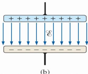
Capacitance is a measure of a capacitor's ability to store charge on its plates.
