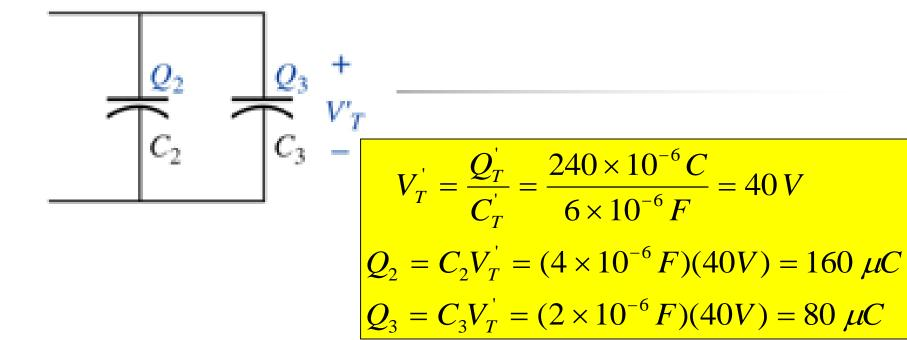
**Example7:** Find the voltage across and charge on each capacitor for the network, after each has charged up to its final value
