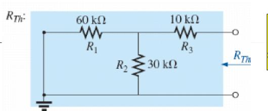
$$= \frac{R_{Th} = (R_1//R_2) + R_3}{\frac{(60k\Omega)(30k\Omega)}{60k\Omega + 30k\Omega}} = 30(k\Omega)$$
