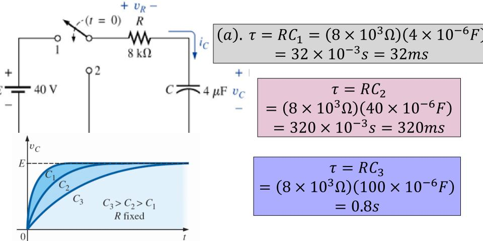
**Example11:** Find the mathematical expressions for the transient behavior of  $v_C$  and  $i_C$  for the circuit when the switch is closed position 1 at t = 0s.
