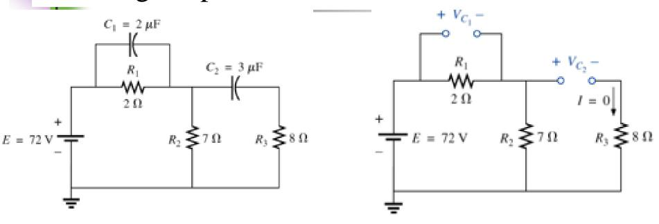
$$V_{C_2} = \frac{(7\Omega)(72V)}{7\Omega + 2\Omega} = 56(V)$$
