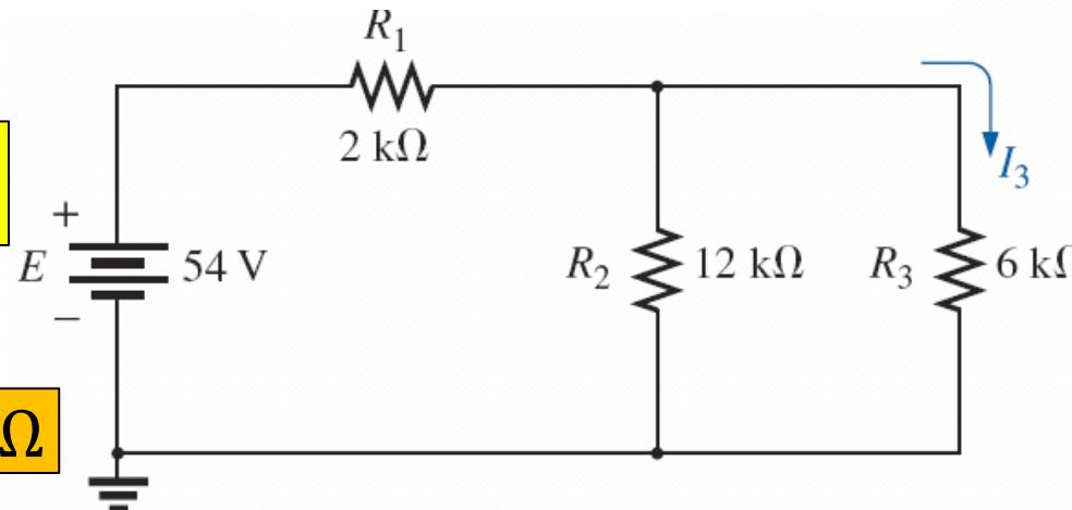
$$R_T = R' + R_1 = 4\text{k}\Omega + 2\text{k}\Omega = 6\text{k}\Omega$$
