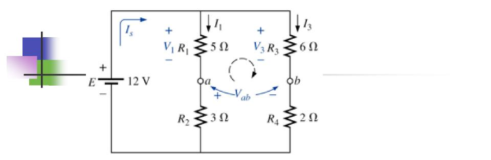
b. By Ohm's law,  $I_1 = \frac{V_1}{R_1} = \frac{7.5V}{5\Omega} = 1.5 A$  $I_3 = \frac{V_3}{R_3} = \frac{9V}{6\Omega} = 1.5 A$
