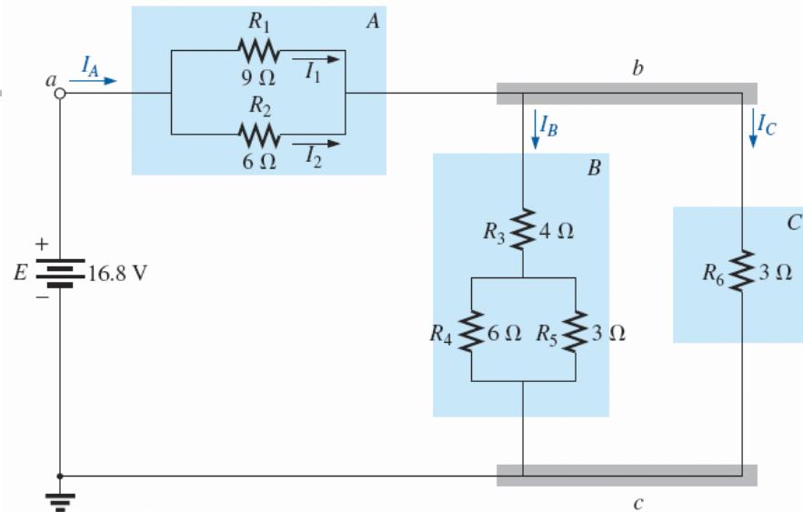
$$R_T = R_A + R_{B//C} = 3.6\Omega + \frac{(6\Omega)(3\Omega)}{6\Omega + 3\Omega}$$
