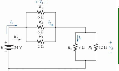
$$I_4 = \frac{V_5}{R_4} = \frac{19.2V}{8\Omega} = 2.4 A$$
