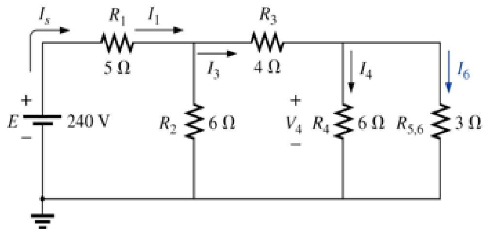
$$I_6 = \frac{(6\Omega)I_3}{6\Omega + 3\Omega} = \frac{6}{9}(15 A) = 10 A$$
