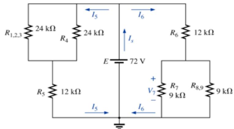
$$I_5 = \frac{E}{R_{(1,2,3)//4} + R_5} = \frac{72V}{12k\Omega + 12k\Omega} = \frac{72V}{24k\Omega} = 3mA$$
