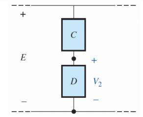
Exp4: Find the current  $I_4$  and the voltage  $V_2$  for the network.
