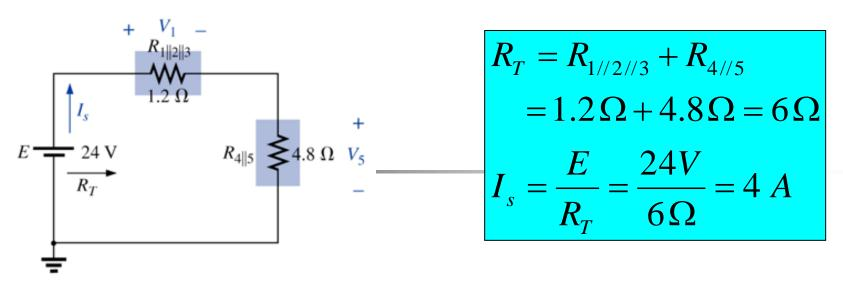
$$V_1 = I_s R_{1/2/3} = (4 A)(1.2 \Omega) = 4.8V$$
