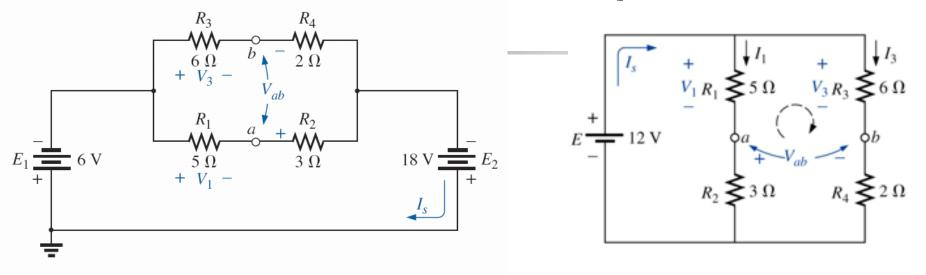
Applying the voltage divider rule yields  $V_{1} = \frac{R_{1}E}{R_{1}+R_{2}} = \frac{(5\Omega)(12V)}{5\Omega+3\Omega} = 7.5V$   $V_{3} = \frac{R_{3}E}{R_{3}+R_{4}} = \frac{(6\Omega)(12V)}{6\Omega+2\Omega} = 9V$ Applying Kirchhoff's voltage law around the indicated loop of Fig.  $-V_{1}+V_{3}-V_{ab} = 0$   $V_{ab} = V_{3}-V_{1} = 9V - 7.5V = 1.5V$
