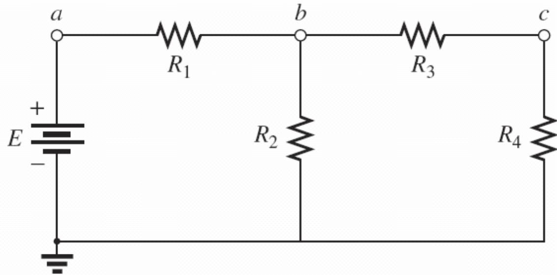
*Series-parallel networks are networks that contain both series and parallel circuit configurations*
