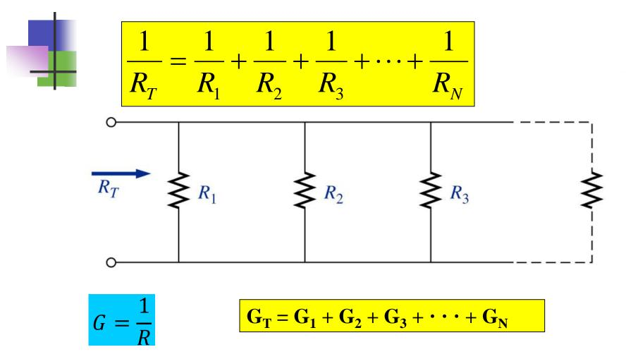
For parallel elements, the total conductance is the sum of the individual conductance.
