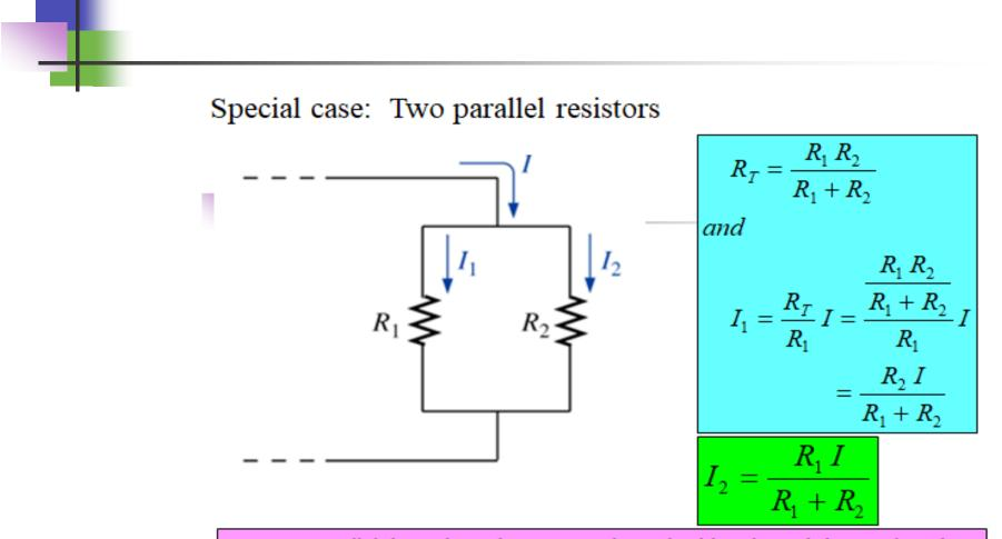
For two parallel branches, the current through either branch is equal to the product of the other parallel resistor and the input current divided by the sum of the two parallel resistances.
