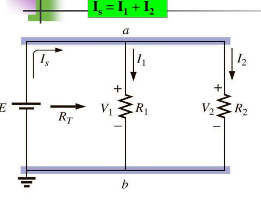
The power dissipated by the resistors is equal to the power delivered by the source.
