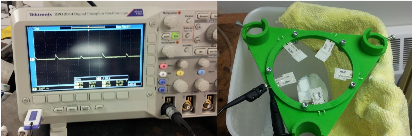
Figure 4.2.1 Piezoelectric testing setup. Shown on left is the oscilloscope used to measure the voltage and current from the piezoelectric. Shown on right is the piezoelectric array with 5 PVDF transducers.
