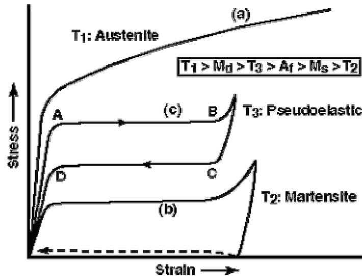
Figure 2.9: Typical stress-strain curves for constant temperatures [2].
