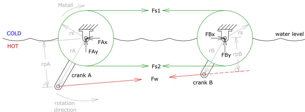
**Figure 4.4:** Forces between a single pair of synchronized cranks. Labels  $r_s$ ,  $F_{s1}$ ,  $F_{s2}$ ,  $F_w$ ,  $F_{Ax}$ ,  $F_{Ay}$ ,  $F_{Bx}$  and  $F_{By}$  represent synchronizer radius, forces in each side of the synchronizer, force in the wire and the x and y-components of force at shaft A and at shaft B, respectively.
