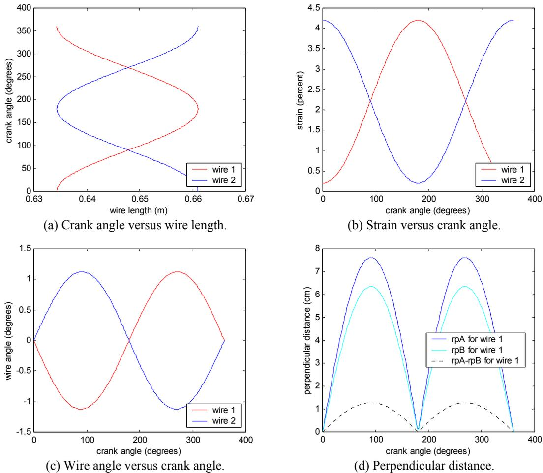
**Figure 4.6:** Plots relating geometric and kinematic quantities for a two-crank synchronized engine ( $r_A = 0.0762$  m,  $r_c = 0.6477$  m,  $\varepsilon_{min} = 0.2\%$ ,  $\varepsilon_{max} = 4.2\%$ ).
