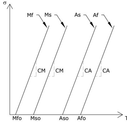
**Figure 2.7:** Transformation temperatures as functions of applied stress.  $M_{fo}$ ,  $M_{so}$ ,  $A_{so}$  and  $A_{fo}$  represent the "original", unstressed transformation temperatures.  $C_A$  and  $C_M$  are stress influence coefficients.
