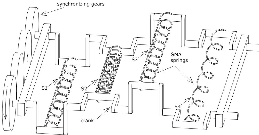
**Figure 3.2:** Diagram of a counter-synchronized twin-crank engine.
