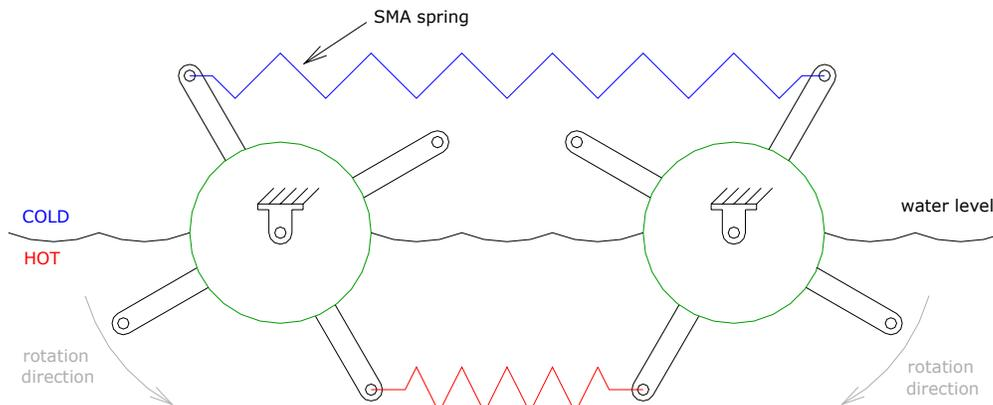
**Figure 3.3:** Simplified end-view of the twin-crank engine.
