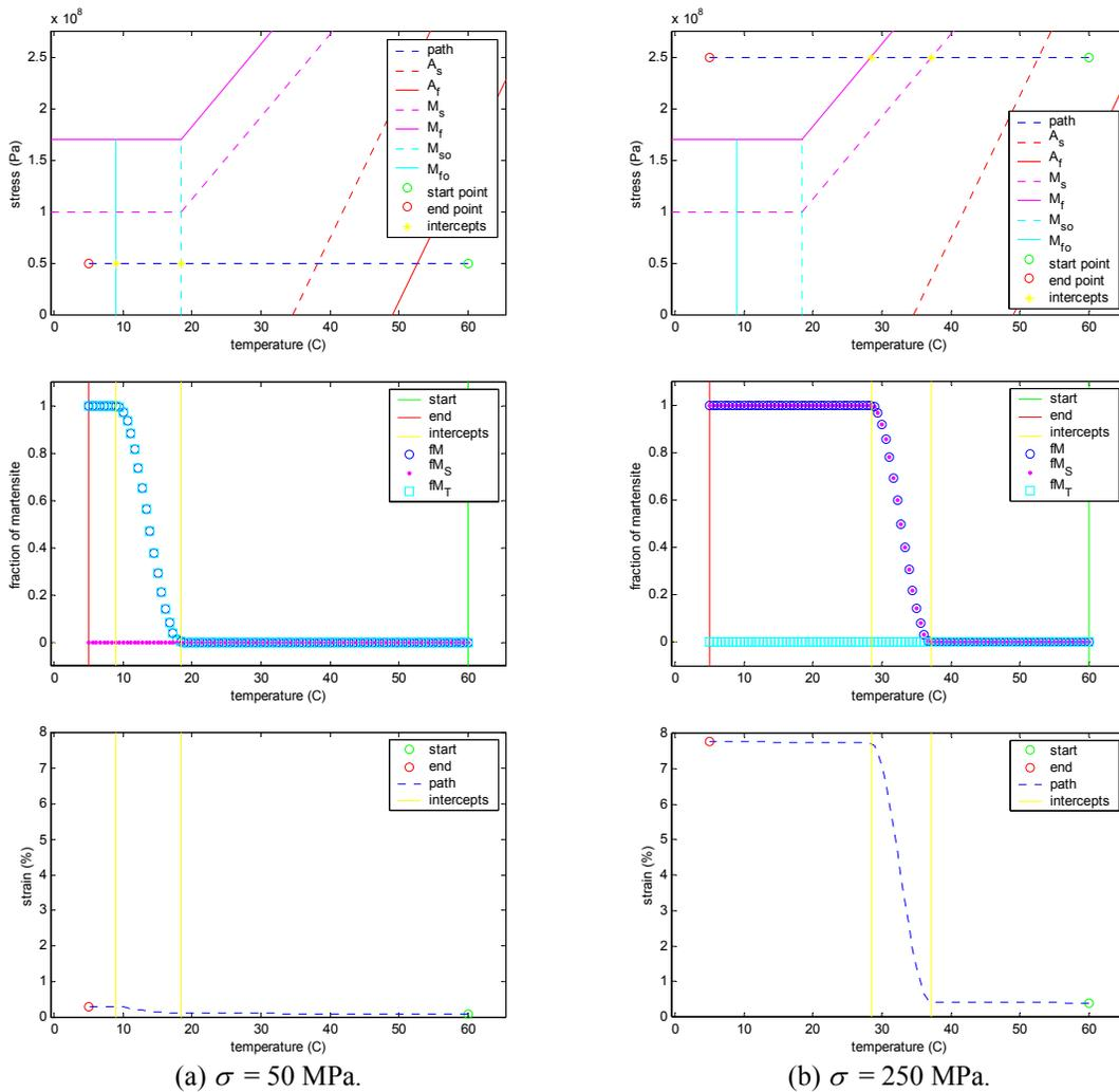
**Figure 2.11:** Path in stress-temperature space, fractions of martensite and strain: (a) constant stress cooling for  $\sigma < \sigma_s^{cr}$ , (b) constant stress cooling for  $\sigma > \sigma_f^{cr}$ .
