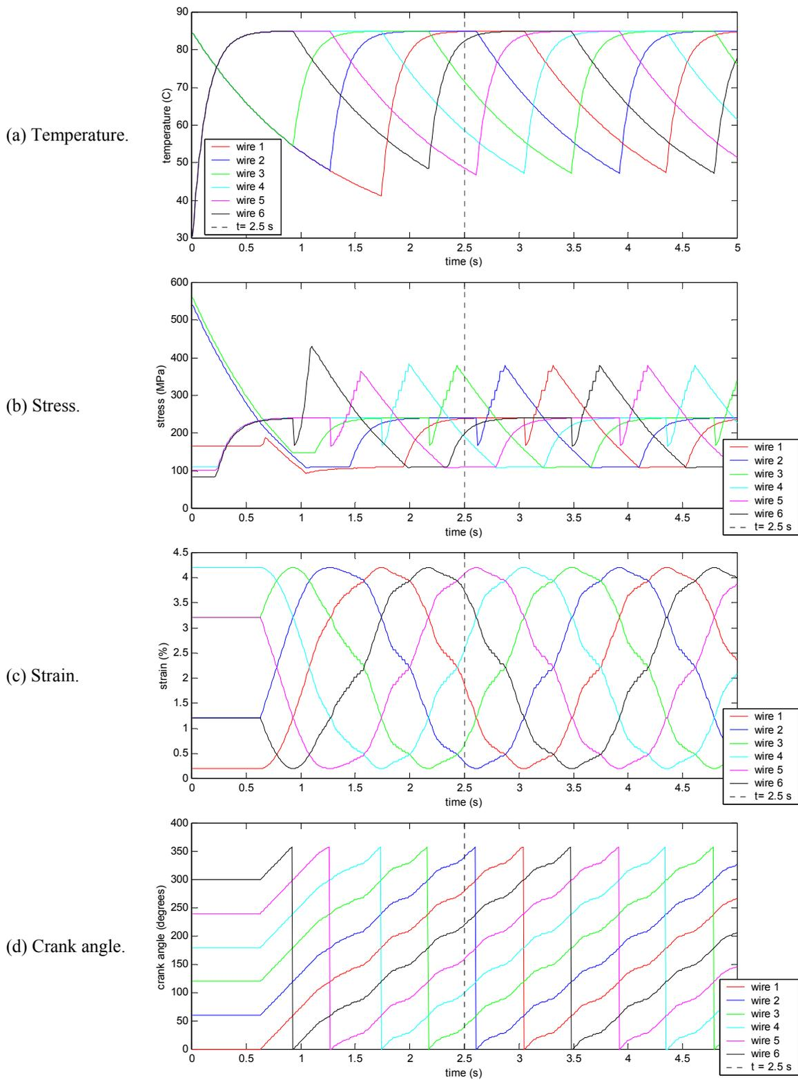
**Figure 4.9:** Simulation results under zero-load, forced convection conditions.
