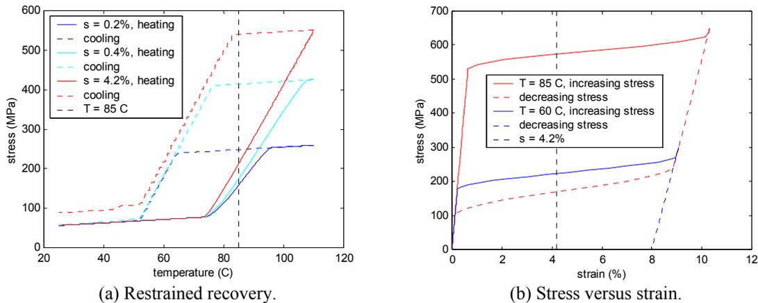
**Figure 4.8:** Constitutive relations: (a) restrained recovery for a series of constant strains, each starting from the same initial stress (b) stress-strain curves at constant temperatures, both starting with zero initial strain.
