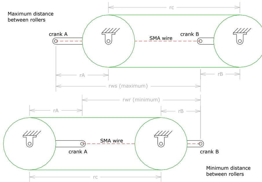
**Figure 4.2:** Limit positions for a pair of aligned cranks. Labels  $r_c$ ,  $r_{ws}$ ,  $r_{wr}$ ,  $r_A$  and  $r_B$  represent center distance, wire length - stretched, wire length - retracted, length of crank A, and length of crank B, respectively.
