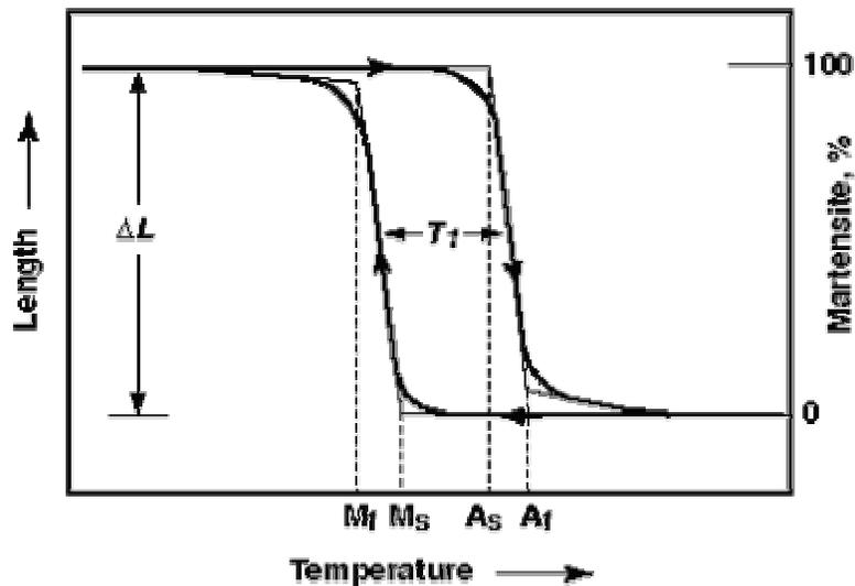
**Figure 2.6:** "Typical transformation versus temperature curve for a specimen under constant load (stress) as it is cooled and heated.  $T_1$ : transformation hysteresis;  $M_s$ : martensite start;  $M_f$ : martensite finish;  $A_s$ : austenite start;  $A_f$ : austenite finish" [2].
