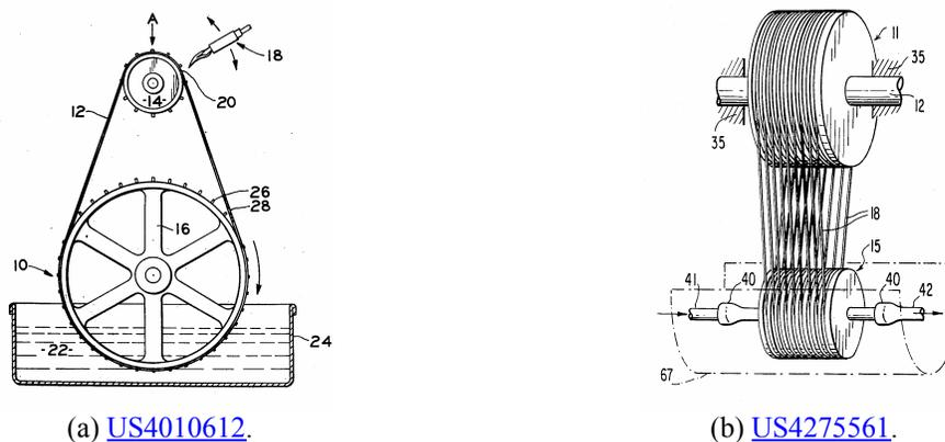
Figure 3.5: Patented unsynchronized pulley engines.
