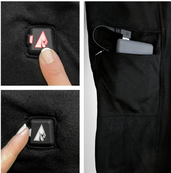
Figure 3: Button used to turn on device as well as control heat settings. Also shows the pocket the powerbank goes in.
