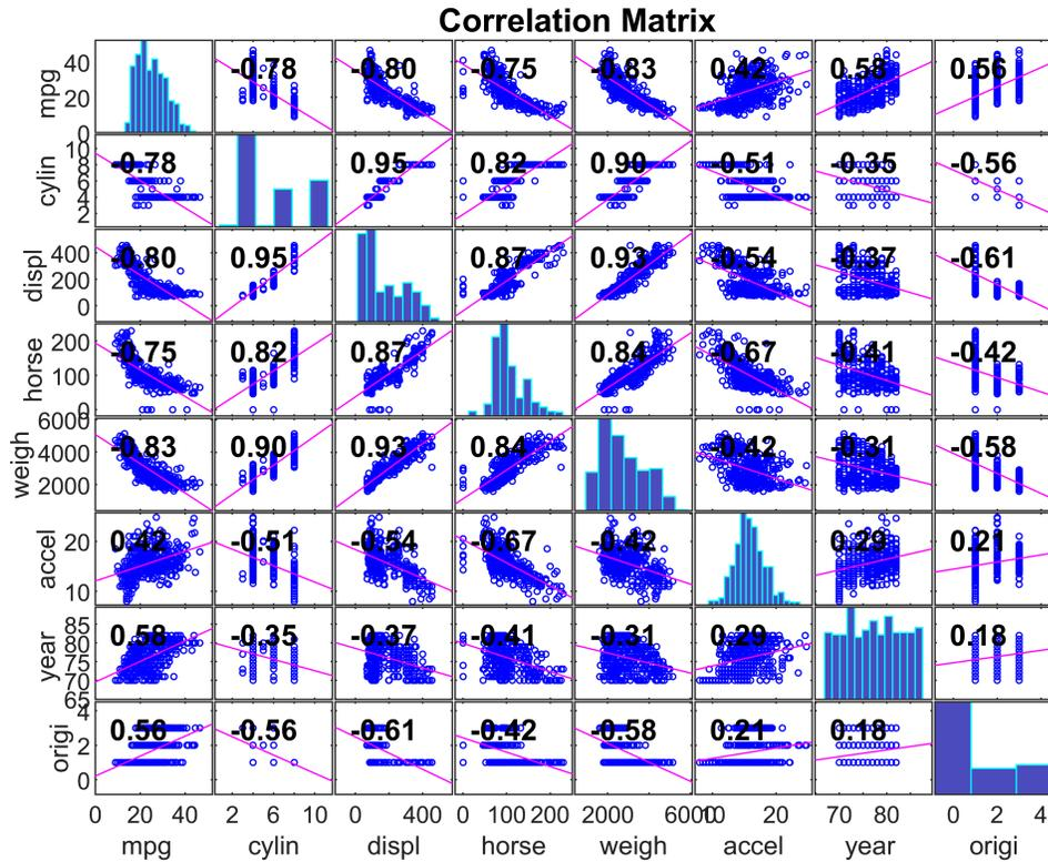
. The goal of this exercise is to see if we can predict the milage (mpg) given the car's other characteristics. From the plot above it seems the columns displacement, horsepower and weight correlate well with mpg. Thus the plan is to make a model that predicts mpg given those three columns.
