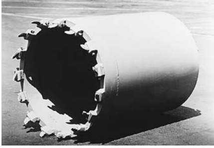
FIGURE 2.39 For cutting through hard material, the caisson drill is equipped with a carbide-toothed coring bucket. (Courtesy of Calweld Inc.)
