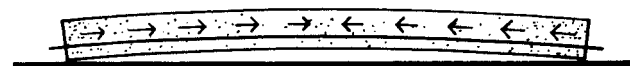
3. When the strands are cut the concrete goes into compression and the beam takes on a camber
