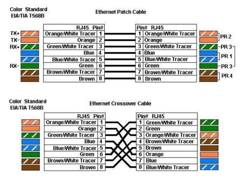
This is the standard color charts of a straight-through and crossover cable. This diagram is used when creating these cables. To make this cable, you will need CAT-5, non-plenum Ethernet wire, RJ-45 (Ethernet) male connectors, wire cutters, and a crimping tool for RJ-45 connection.
