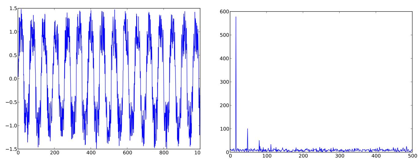
A periodic function with some noise. Taking the Fourier transform and plotting it as a power spectrum we can see the signal is primarily at one frequency with some power at harmonics as twice, three and four times the fundamental frequency. We can also see white noise, white because it has roughly the same amplitude at different frequencies. We could filter out the noise by performing the inverse DFT, but only for the 4 or 5 largest Fourier coefficients.
