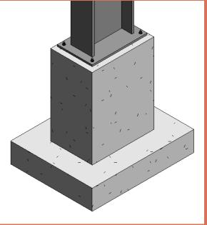
Column Base Plate to Isolate Footing
