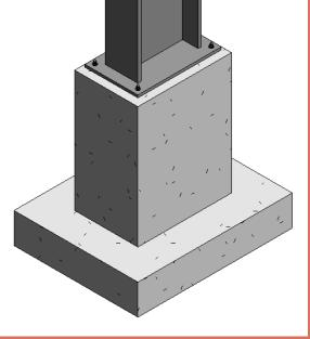
Column Base Plate to Isolate Footing
