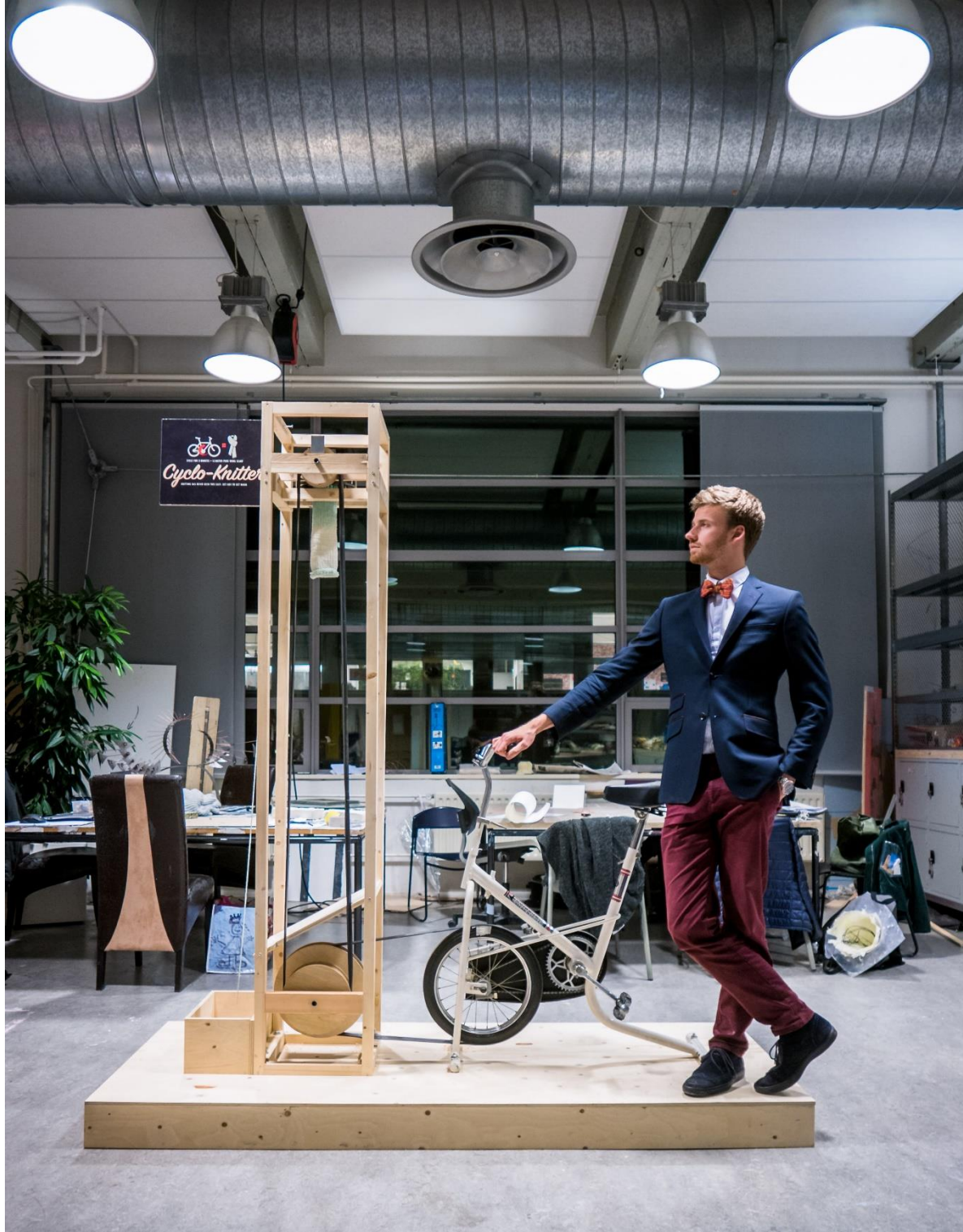
Fig. 2: Bike - Powered Scarf Knitter / Cyclo - Knitter by George Barrat - Jones.
