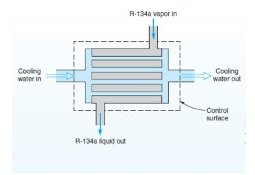
$$m_{r}(h_{1}r + m\omega(h_{1})\omega = m_{r}(h_{e})r + m\omega(h_{e})\omega$$
