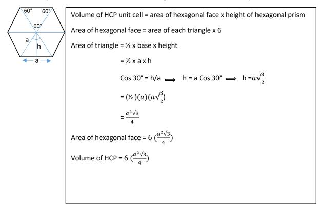
(b). Berilum (Be) has an HCP unit cell for which the ratio of the lattice parameters c/a is 1.568. If the radius of Be atom is 0.1143 nm. (a) Determine the unit cell volume and (c) Calculate the theoretical density of Be.
