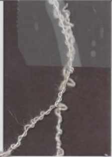
Sample N42 / ratiné yarn / 100% rayon / ratiné (loop) yarn / irregular loops along length of yarn
