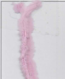
Sample N31 / chenille yarn / 100% nylon / synthetic fibers / chenille yarn / nylon is highly resilient, thus a good choice for pile yarns / fuzzy yarn
