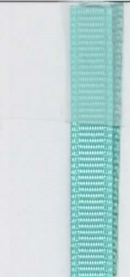
Sample N45 / crossgrain ribbon / 100% polyester / unbalanced heavyweight woven fabric / rounded rib / narrow fabric
