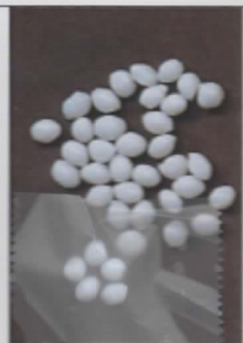
Sample N32 / polyester resin / 100% polyester / synthetic fiber / polyester is the most widely used fiber overall / courtesy of DAK Americas www.dakamericas.com
