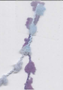
Sample N43 / spot yarn / 100% microfiber polyester / spot yarn a.k.a. knot, nub, or knop yarn
