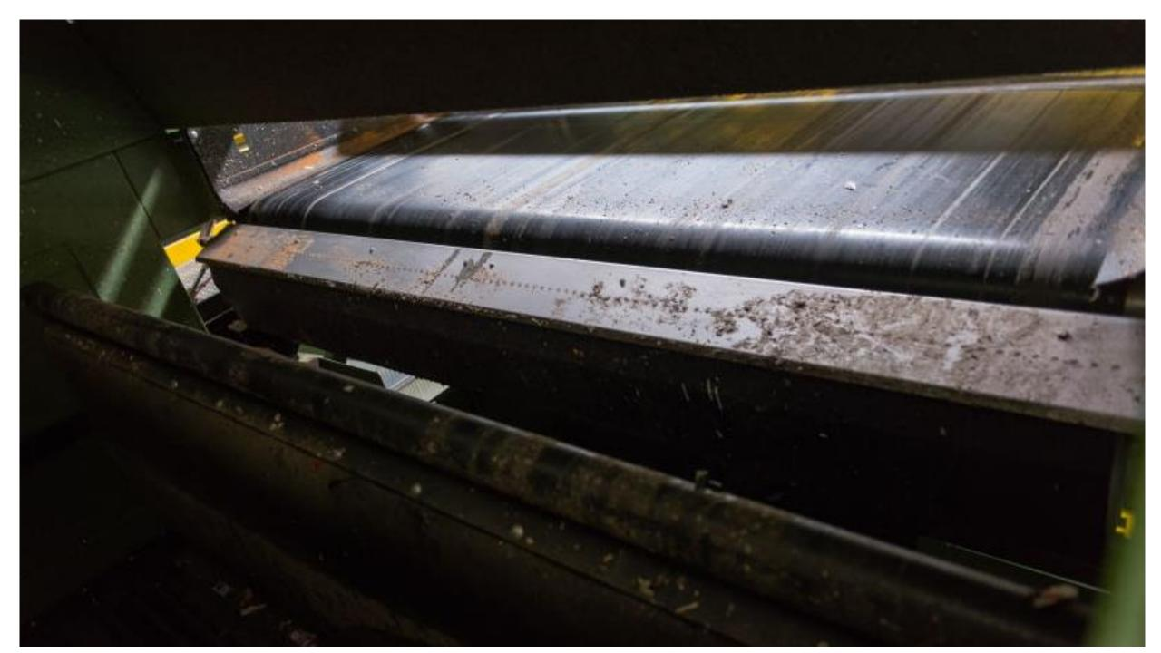
The massive drum shaped machine removes tin cans from the rest of the materials and sends them to a baler.
