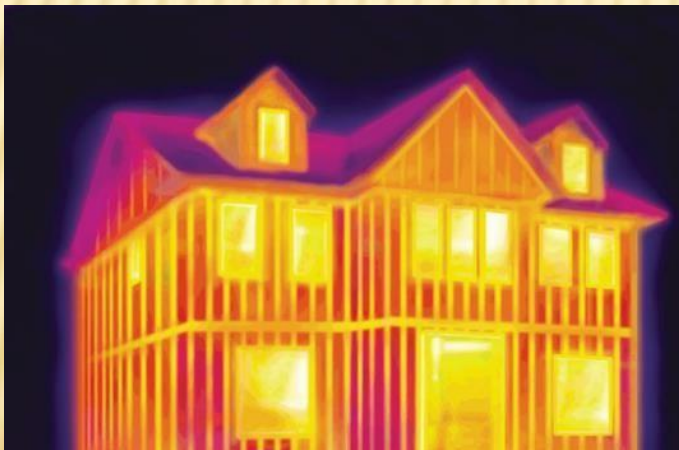
Insulation in between framing
