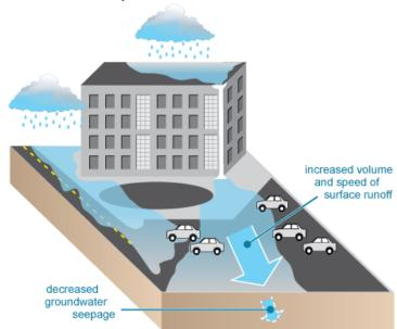
Impervious 'hard' surfaces (roofs, roads, large areas of pavement, and asphalt parking lots) increase the volume and speed of stormwater runoff. This swift surge of water erodes streambeds, reduces groundwater infiltration, and delivers many pollutants and sediment to downstream waters.
