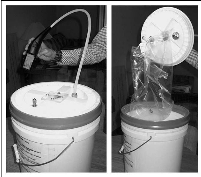
Figure 2. Bucket, as Typically Deployed (Left), and Open to Show Tedlar Sampling Bag (Right)Source: Photos by author
