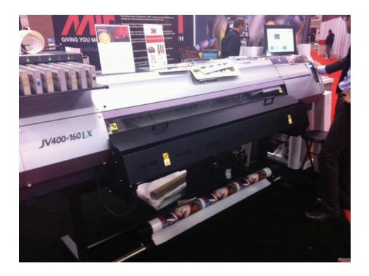
Here is the actual Digital Printer from Mimaki. This printer is 60 inches wide. it has 8 solvent ink cartriges. It has what we know as CMYK & Light ones due to a better color display once any graphic is printed. The features of this printers are amazing. Not only because is Wide large, but it could take several materials as fabrics, canvas, vynils, banner, ecxotic, photo paper, coated and uncoated.
