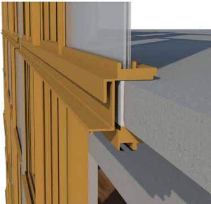
DETAIL AT FLOOR SLAB
