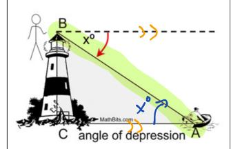
In this diagram,  $x^{o}$  marks the angle of depression of the boat at sea from the top of the lighthouse.
