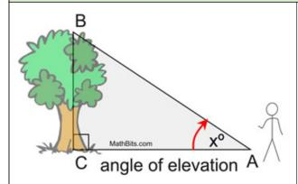
In this diagram,  $x^0$  marks the angle of elevation of the top of the tree as seen from a point on the ground.
