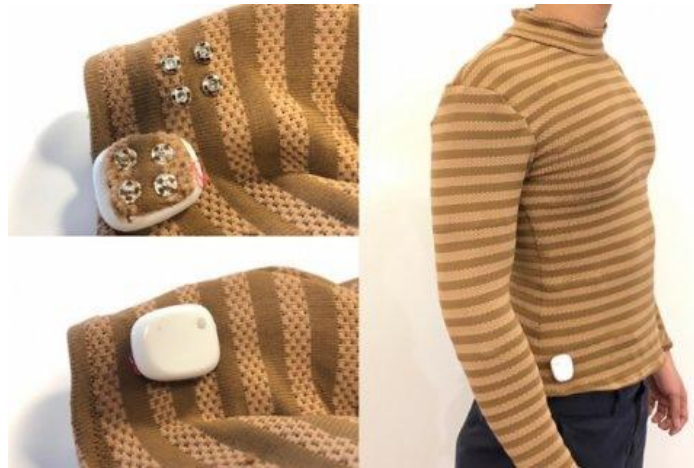
Figure 3: Sensors woven into a shirt can monitor vital signs
