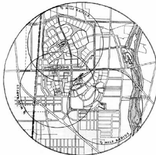
General plan showing neighborhoods. Stein, Clarence S. Toward New Towns for America . 1957. Cambridge: The MIT Press, 1989. 50.
