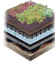
Extensive green roof
