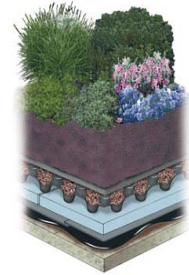
Intensive green roof
