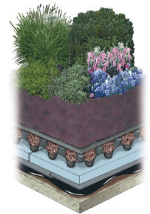
Intensive green roof
