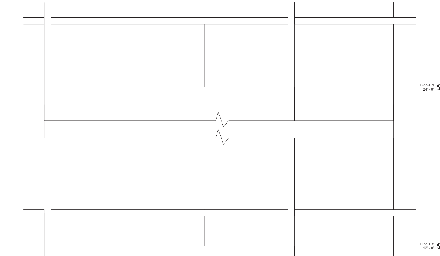
ELEVATION OF A UNITIZE CURTAIN WALL SYSTEM ① WALL SYSTEM 1 1/2" = 1'-0"
