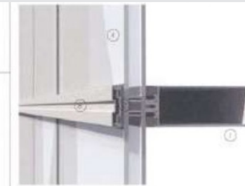
Basic capped unitised glazing detail
