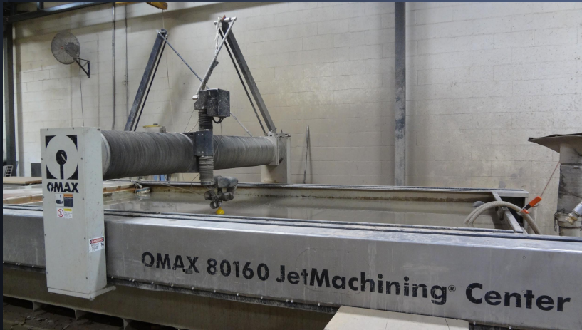
The OMAX 80160, Bed 14' 6" X 7' 5", 30HP/45, 000PSI. Accuracy of up to .0135 " (less than 1/64")
