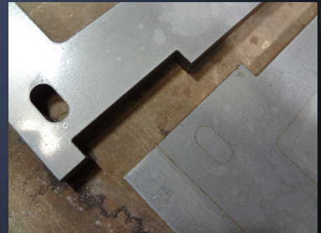
Right. The material pictured is \frac{1}{8} " thick aluminum. Notice the precision and clean cuts of the shapes cut out of the metal.
