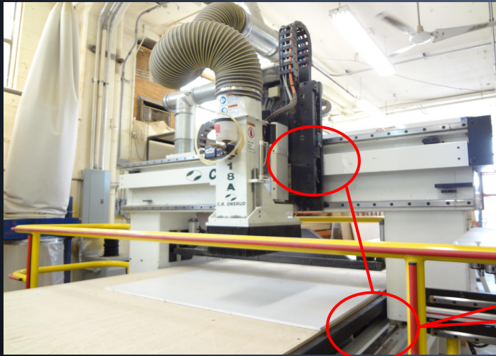
The Onsrud 145G18A used at Scenic Corp Specs: 5' X12' Bed, 18HP/18000RPM Spindle, 12 tool automatic changer.
