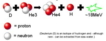
The University of Wisconsin-Madison's Fusion Technology Institute ("TCI") developed technology needed to pair deuterium with Helium3, trigger and then sustain a fusion reaction. The result is a "high-energy proton (positively charged hydrogen ion) and an alpha particle (4He ion) for a total kinetic energy of 18.4 MeV."
