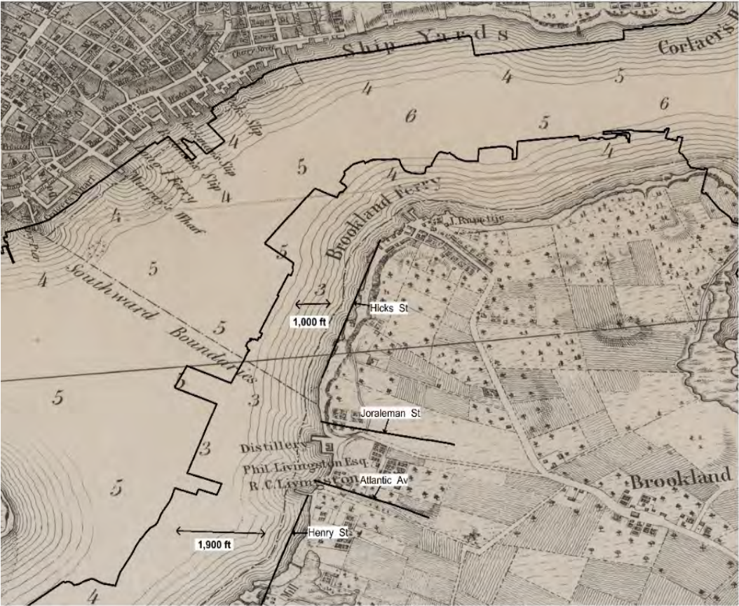
Map 1 Brooklyn & Manhattan Waterfront: “Made-Land” 1776 British Naval Map & Current Shoreline Source: NYPL MapWarper - 1776 Blaskowitz British Navy map; NYC Planning - shoreline
