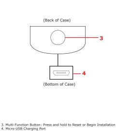
Charging the Case Insert the small connector of the supplied micro-USB charging cable into the micro-USB charging port on the back of the charging case. Insert the large connector into the USB port on a computer, a USB charging device, or 5V USB adapter (not included) and plug into a wall socket. The case-charging LED indicator will flash RED while charging and turn solid GREEN when fully charged.
