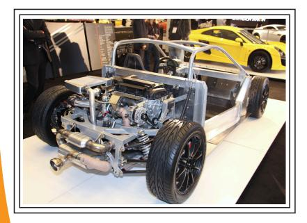
**The Mastretta** is the first car fully designed and built in Mexico. The car we're driving today is very much a pre-production prototype; it's powered by a Volkswagen TFSI engine, whereas the production cars will have a turbocharged Ford Duratech motor with around 238bhp. The whole car is targeted to weigh 900kg, which puts it right on a par with the Elise. Lifestyle Cars, which is the European importer, pitches the car in a gap between the Exige and Noble.
