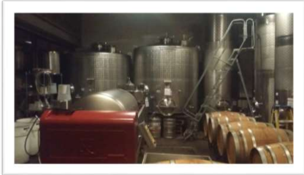
Large stainless steel fermentation tanks, crusher/destemmer (red), pneumatic press (sideways cylinder)
