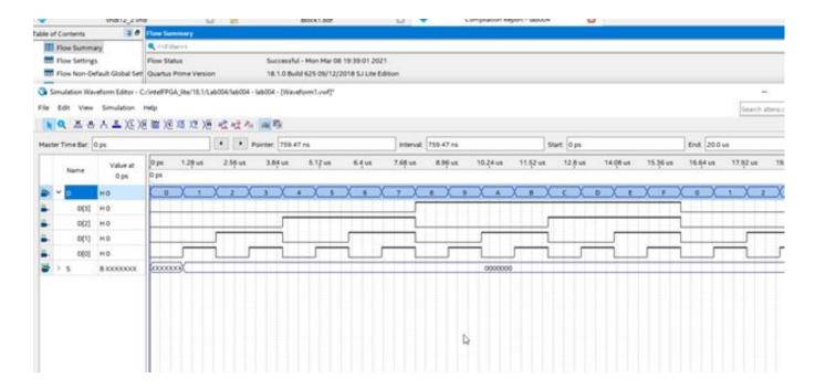
Each wave represents your input for your design, when your waveform is low, this will represent a logical 0 in your program. When the waveform is high this represents a logic 1 in your program. Together D[3] - D[0] will represent a number each count as shown below.
