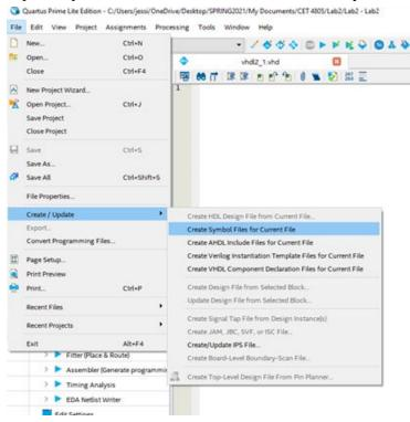
5. Open a new Schematic file (**File>New**) by highlighting **Block Diagram/Schematic File**. And click **OK**. And construct the circuit using the symbols you just create. Each symbol should be available in the Project Library in the Symbol diagonal box.
